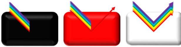
Figure 1. How objects with different color reflect incident white light
